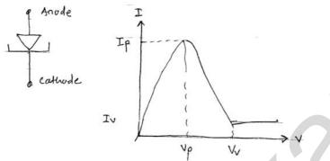
The Tunnel diode is a specially made P-N junction diode which exhibits negative Resistance over part of the forward characteristics. It has extremely heavy doping on both sides of junction and abrupt transition from P-side to the n-side. The Tunneling effect is a majority carrier effect and is consequently very fast.
