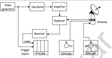
Fig.2 : Block diagram of pulsed radar
