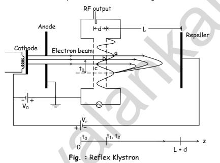
The electrons a shown in figure which leave the gap at positive half cycle of the RF field in the cavity gap d will be accelerated. While electrons b travel with unchanged original velocity, and the electrons c will be retarded on entering the repeller space.
