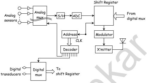
Fig.1: Block diagram of telemetry unit
