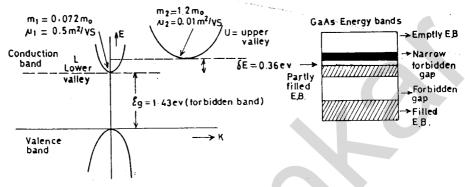
Basic mechanism involved in the operation of bulk n-type GaAs device (gunn diode) is the transfer of electrons from lower conduction valley (L-valley), to upper subsidiary valley (U-valley). This concept of Electron transfer is also known as "Gunn effect".
