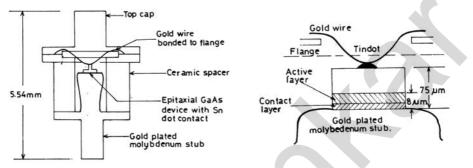
Gunn diodes are grown epitaxially out of GaAs or InP doped with silicon. The substrate, used here is highly doped for good conductivity, while the thin active layer is less heavily doped. The gold alloy contacts are electro deposited and used for good ohmic contact and heat transfer for subsequent dissipation.
